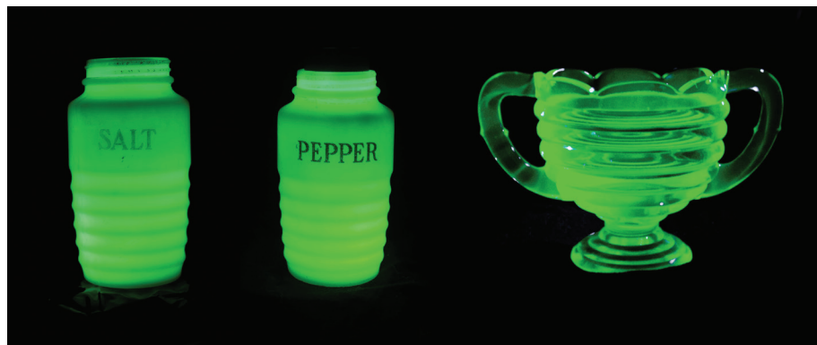
Figure 3. Uranium luminescence observed as a green glow when exposing the uranium-impregnated glass to UV light. Photo courtesy of Kirstie and John Ahern.
