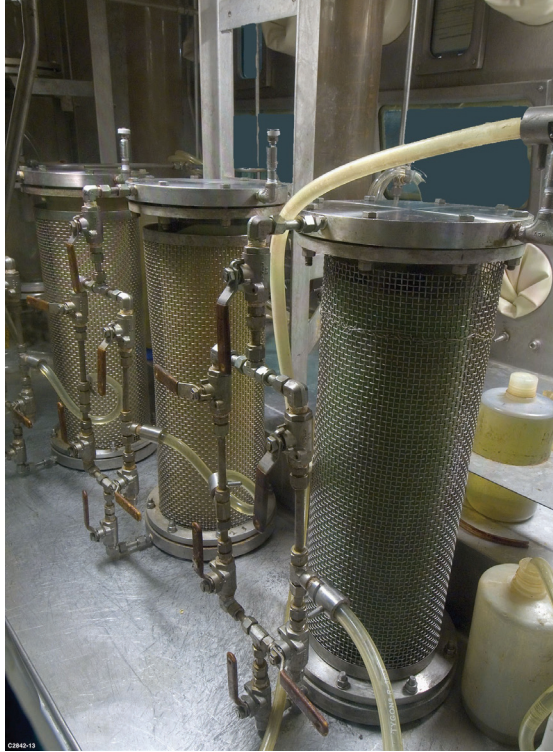
Figure 2. Anion exchange resin columns used in aqueous nitrate processing.
